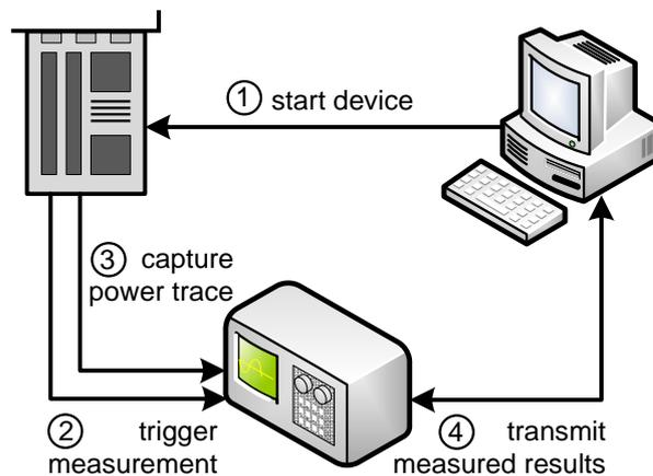
Figure 13: Setup for a power analysis attack
