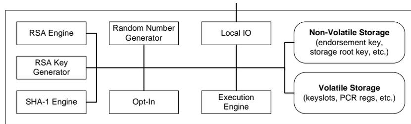
Figure 10: Block diagram of a Trusted Platform Module (TPM)
