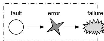
Figure 2: Fault model after [85].
