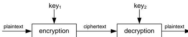
Figure 9: *Cryptosystem: Principle of Operation*
