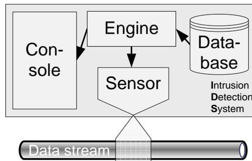
Figure 7: Block diagram of intrusion detection system
