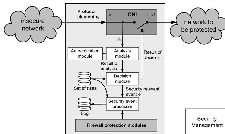
Figure 6: Structure of a firewall element connecting a secure and an insecure network
