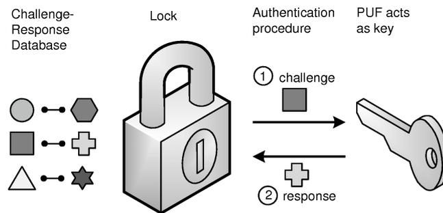
Figure 12: How a PUF can be used as an uncloneable key.
